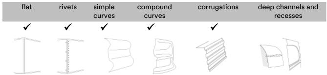
**Important Notice:** Application on corrugations should be done by following the shape without stretching the film. Inlays and relief cuts in deep recesses are recommended.
